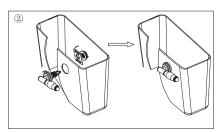
Install the lever in the front hole and fix the nut properly.
