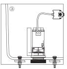
Nest the Tank To Bowl Washer in the Lock Nut and position the TANK on the Toilet Bowl properly. Disassemble the Tank To Bowl Bolts. Fix the Tank to Toilet Bowl with the Tank To Bowl Bolts tightly.
