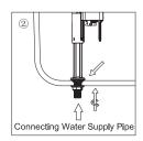
Position VALVE inside tank. Twist the Valve Shank clockwise, and pull the Valve Body to an expected height, and then twist the Valve Shank anticlockwise to fixed it.
