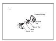
Unlock the Button Fixer of claw housing, take out the front lever, then loosen the lever nut.
