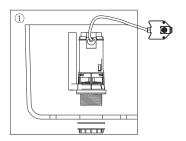
Disassemble lock Nut for Valve installation. Position the VALVE inside the TANK. Push down on the Valve Body while tightening the Hexagon Nut from outside.
